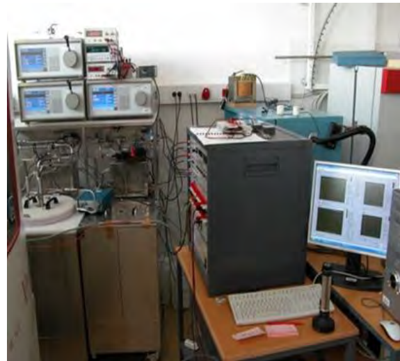
Figure 1: The LMK primary dew-point generator, which represents a national reference for humidity measurements
